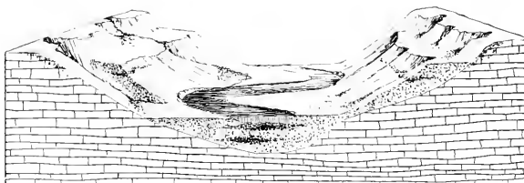
FIG. 26. Diagram showing how a river may destroy terraces by side cutting.
